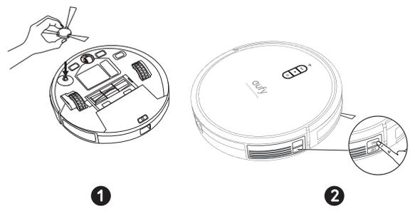
**T** Remove the sticker next to the power switch, and the foam blocks beside the bumper before use.
