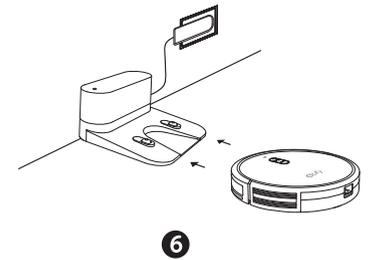
**T** Fully charge RoboVac before use. The LED indicator on the ►|| button breathes orange while charging, and turns solid blue when fully charged.
