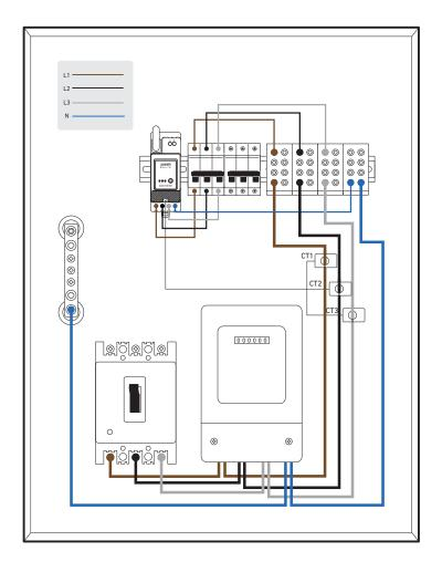
1. Please first identify the entry phases. Under normal circumstances, the brown phase is live wire L1, the black phase is live wire L2, the gray phase is live wire L3, and the blue phase is the neutral wire N.
