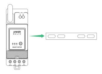
5. Please prepare the corresponding color voltage wire, then connect the voltage wire from any unused circuit breaker hole and connect it to the hole of the corresponding Smart Meter.
