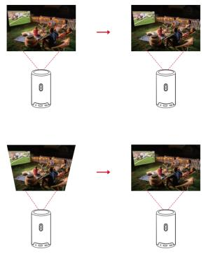
To enable autofocus and auto keystone correction, slightly move the projector or press (a) on the remote.
