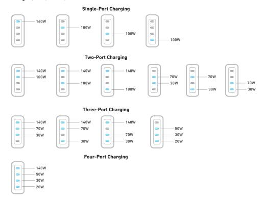
Connect the charger's USB-C1 port to a 16" MacBook Pro using a USB-C to MagSafe 3 cable to achieve a power output of 20V=5A or 28V=5A per port. Similarly, USB-C2, USB-C3, or USB-C4 can each provide a maximum power output of 20V=5A when using the same cable.
