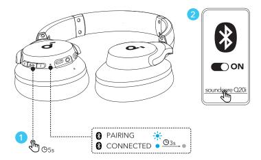
To manually enter Bluetooth pairing mode, power off the headphones and press the multi-function button for 5 seconds.
