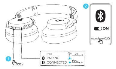
Press and hold the multi-function button for 2 seconds to power on. The headphones will automatically enter Bluetooth pairing mode when connecting for the first time.
