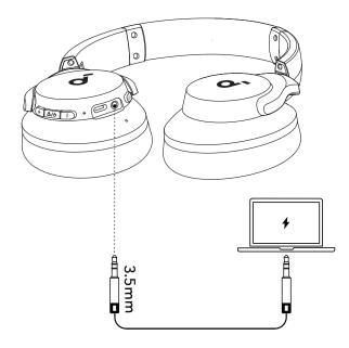
Play audio on an external device by plugging in a 3.5mm AUX cable. Wired listening will automatically turn off Bluetooth mode.
