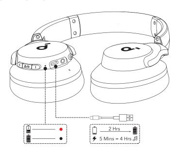
Fully dry off the headphones and USB-C charging port before charging. Do not turn on your headphones while charging. Use a certified USB-C charging cable and charger to prevent any damage.
