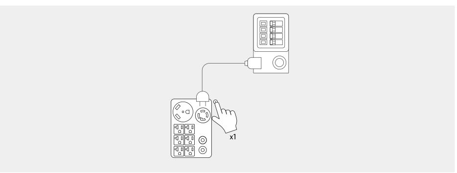
2. Double-press the AC outlet button to turn on EV mode, wait until the car icon appears on screen, then connect your device to the L14-30R AC output port. When the power station is in EV Charging mode, it cannot be charged via AC simultaneously.
