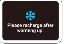
Temperature Protection Mode: Activates when the battery temperature is too high or too low, suspending the operation of the power bank until the temperature normalizes.
