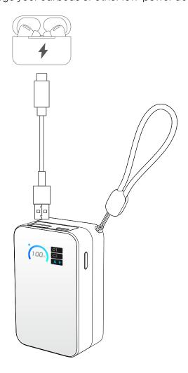
3. Press the power button twice to deactivate trickle charging mode. Trickle charging mode automatically turns off after 2 hours if the USB-A port is not in use.
