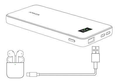
3. Press the button twice to exit trickle-charging mode.
