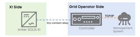
Currently, All Anker SOLIX XI Single-Phase/Three-Phase Energy Storage System supports EnWG14a.
