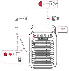
Plug the cord into the adapter. Then connect the projector to the power supply. When successfully connected to the power supply, the power button on the projector will turn red.
