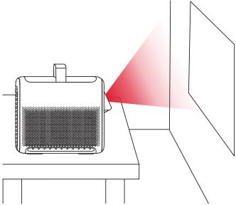
The built-in micro gimbal adjusts the projected image position automatically during Spatial Adaptation.
