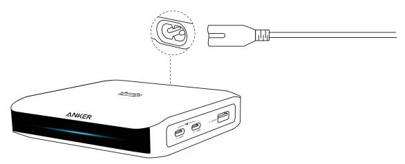
Charge your devices via the USB ports. The indicator light will flash twice when a new device is connected.
