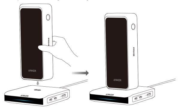
To remove the power bank, tilt it slightly backward and lift it up.
