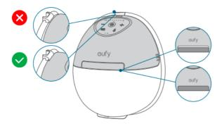
The locking mechanism between the pump hub and the pouring spout ensures reliable suction.
