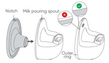
3. Insert the diaphragm into the groove of the container, with the concave side of the diaphragm facing the flange side.
