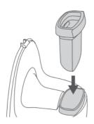
4. Install the pump hub on the top of the container, pressing firmly to seal the gap between the pump hub and the diaphragm.
