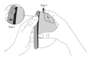
The locking mechanism between the pump hub and the pouring spout ensures reliable suction.
