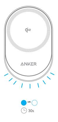
If input power is below 18W, charging will pause and the ambient light will flash slowly (once per second). Use an adapter or USB-C port with at least 45W input for better performance.
