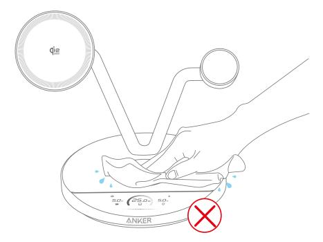
Adjust the position of your devices to align them properly with the charging surface. Remove any metal objects between your device and the charger to maintain proper charging performance.
