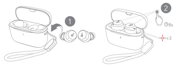
Reset if the earbuds have issues pairing with each other or with other devices. Place the earbuds in the charging case and leave the case open, then tap and hold the touchpads on both earbuds for 8 seconds until the earbuds' LED indicators flash red rapidly three times.
