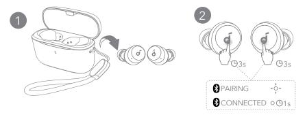
To manually enter Bluetooth pairing mode, take the earbuds out of the case, then tap and hold the touchpads on both earbuds for 3 seconds until the earbuds' LED indicators flash white rapidly.
