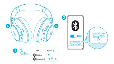
Press and hold the power button for 2 seconds to turn on. The headphones will automatically enter Bluetooth pairing mode when connecting for the first time.
