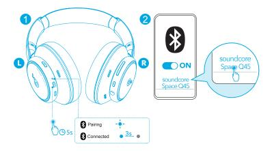
To manually enter Bluetooth pairing mode when the headphones are off, press and hold the power button for 5 seconds until the LED flashes blue.
