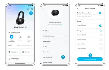
In the soundcore app, go to settings and select **Dual Connections** > **Connect New Device.**
