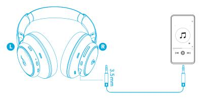
Play audio on an external device by plugging in a 3.5mm AUX cable. Wired listening will turn off Bluetooth mode automatically.
