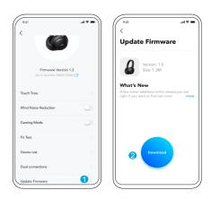
You will be informed once the new version of firmware is detected when you connect the headphones with the app. Ensure the headphones are powered on and connected to a device until the firmware update is complete. During the update, avoid any usage and ensure stable access to the internet.
