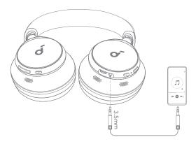
Play audio on an external device by plugging in a 3.5mm AUX cable. Wired listening will automatically turn off Bluetooth mode.
