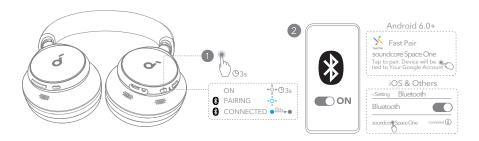
**Auto Pairing:** Press and hold the power button for 3 seconds to power on. The headphones will automatically enter Bluetooth pairing mode when connecting for the first time. Select "**soundcore Space One**" on your device's Bluetooth list to connect.
