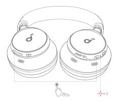
You might need to reset your headphones if you experience connectivity or function issues. Delete the pairing history from your Bluetooth device first. Press and hold the volume up and power button simultaneously for 5 seconds until the LED flashes red three times.
