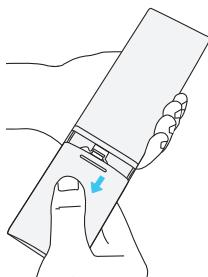
② To replace the batteries, slide off the battery compartment backplate, insert new batteries (matching the polarity (+/-) as indicated), and close the battery compartment.
