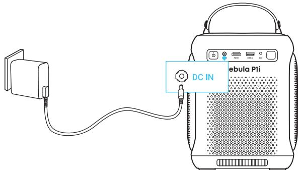
Connect the adapter to the power and attach the DC plug to the projector.
